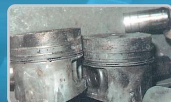
Burned pistons and rings resulting from carbon deposit and knock caused by incomplete combustion.
